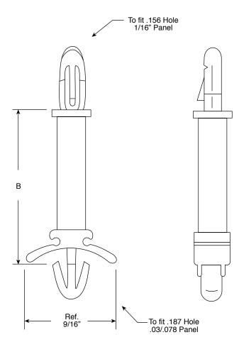
Circuit Board Supports eliminate screws, nuts, and lockwashers in mounting printed circuit boards on metal chassis or stacking in multiple tiers. Unique locking designs provide mechanically secure, reusable connection in predrilled or punched holes while saving considerable assembly time and expense. The LLP Series is designed to securely lock both the chassis end and the printed circuit board on top.
